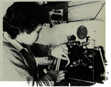
1. This Bell & Howell 16 mm continuous contact wet motion picture printer which has an automatic additive color light source with microprocessor color/frame count cue memory system.
