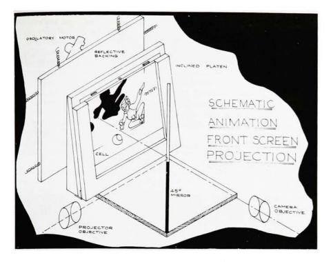
for the utmost stability and erected in an entirely black painted room to eliminate any spurious reflections of objects in the glass and mirror surfaces of the apparatus.
