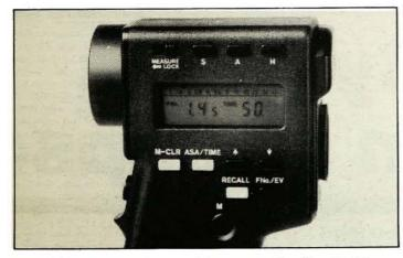
Finally, Minolta technology is available to cinematographers, with the new 1/50th second speed. Minolta digital displays calibrate to within 1/10th of a stop and the analogue display allows for memory and averaging. Precise adjustment of  $\pm 1$ EV allows you to fine tune your exposure to equipment or film stock variables. Come in today for a demonstration of the Auto Meter III, the Color Meter II or the Spotmeter M.
