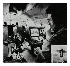
and tilt up or down 46 deg. With the addition of a TV camera taking only 15% of the light from the relay lens, the system can be operated by the cameraman with a joystick while watching a television monitor. Astrovision also has an office in London, England, at 54 Curzon St.
