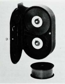
As the film unwinds from the feed spindle, space is provided for film buildup on the take-up spindle for nearly twice as much film as in a magazine using standard daylight loading spools. Gate rollers provide for a light trap permitting magazine attachment to camera for daylight threading. It has a manual type footage counter which indicates remaining footage. For more information contact: Instrumentation Marketing Corp., 820 South Mariposa Street, Burbank, California 91056.
