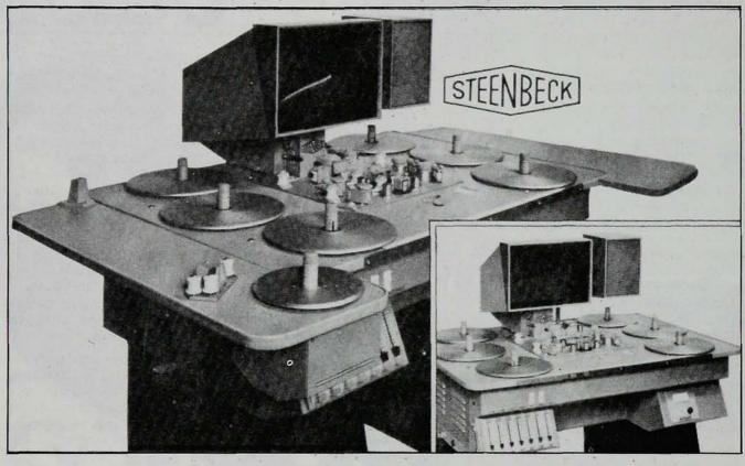
Ideal for those small spaces...this table is only 43" wide. Yet it's a complete 16 mm editing machine with 6-plates consisting of 2 sound and 1 picture track. This machine also offers edge or centre track heads. 12-watt amplifier and speaker. Counter in footage or minute/seconds. Or choose the model with table top extensions
